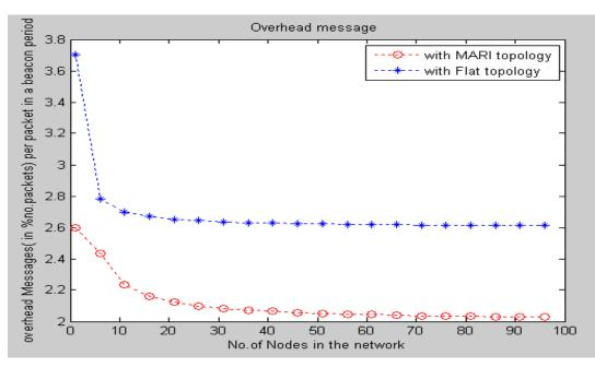
Fig. 5: overhead in each packet per node
