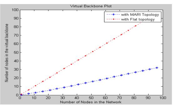
Fig.4: Number of nodes in the backbone as the number of nodes in the network increases
