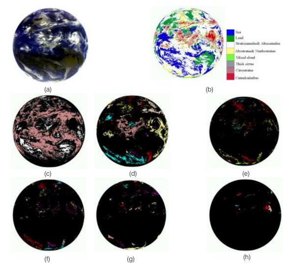
*Fig.3:* (a) pseudo-color composite map of Tbb of IR1, IR2 and WV(16: 00 UTC on 9 July2007); (b) cloud classification results of ANN ;(c) Segmentation result of low cloud; (d) Segmentation result of medium cloud; (e) Segmentation result of thin cirrus; (f) Segmentation result of thick cirrus; (g) Segmentation result of multi-layer cloud; (h) Segmentation result of cumulonimbus.
