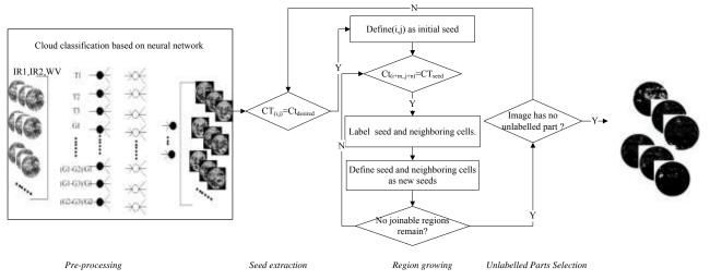
*Fig. 1:* Configuration for the cloud segmentation; CT<sub>seed</sub>-Cloud type of seed; CT<sub>desired</sub>-Desired cloud type; CT<sub>i, j</sub>-Cloud type of pixel (i, j).
