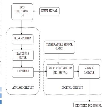
Fig.2: Block Diagram of ECG Device
