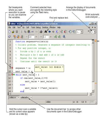
Figure5: M-file debugging-edit function
