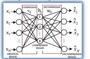
Fig. 1-Basic image compression structure using neural network
