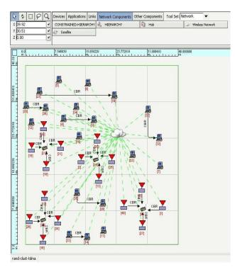
Fig.4.Random topology scenario with Conventional TDMA
