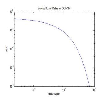
Fig.3 shows the relationship between the bit error rate and  $E_b / N_o$  simulated in Matlab. The bit error rate decreases when  $E_b / N_o$  increases. The noise power spectral density increases when collision increases. As the number of WLAN sources increases, the BER of IEEE 802.15.4 increases because contentions among multiple WLANs increase the channel usage and cause collisions, which is more powerful interference, source to.
