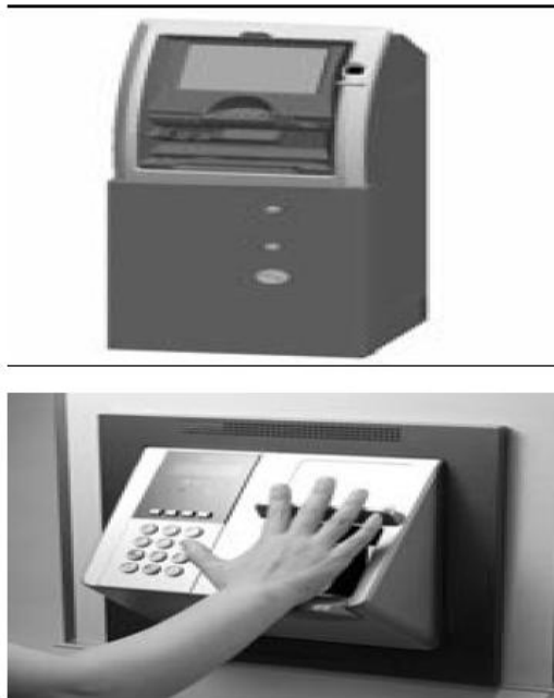
Figure 3. ATM with palm vein access control unit pattern authentication sensor unit
