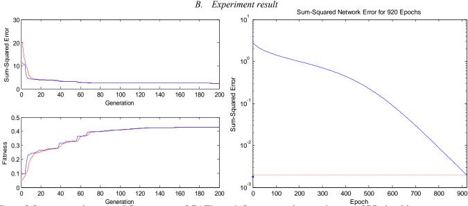
Figure 3:Sum-squared error and fitness curve of GAFigure 4: Sum-squared network error of BP algorithm
