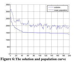
The result shows the sequence of each job, and makespan is 1395 from figure 5. The makespan is attained 1395, when the iterative number is 80, and the mean population is randomfrom the figure
