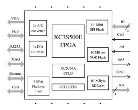
Fig. 10. Artificial cell block diagram
