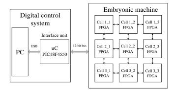
Fig. 12. The hardware system block diagram
