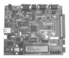
Fig. 11. Spartan-3E Starter KIT development board [13]
