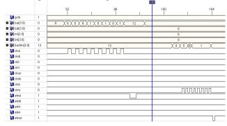
Fig. 14. Network communication waveforms (example\_1)
