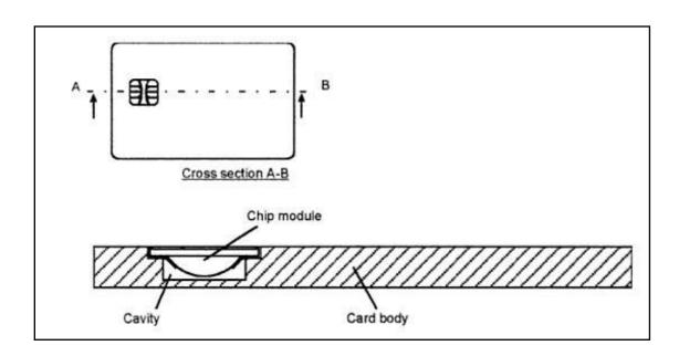
Figure 5: Schematic of Contact smart card
