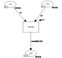
Fig. 4. CPN model of a NAND GATE.
