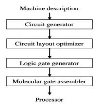
Fig.2. Organization of a nanotechnology-based processor generator.
