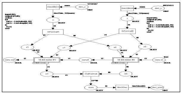
Fig. 6. CPN model of a 32-bit Adder
