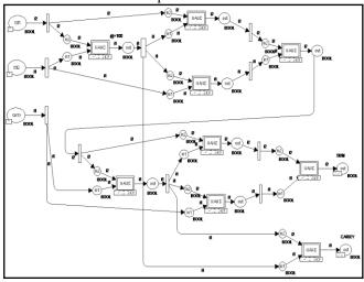
Fig. 5. CPN model of a 1-bit Adder.
