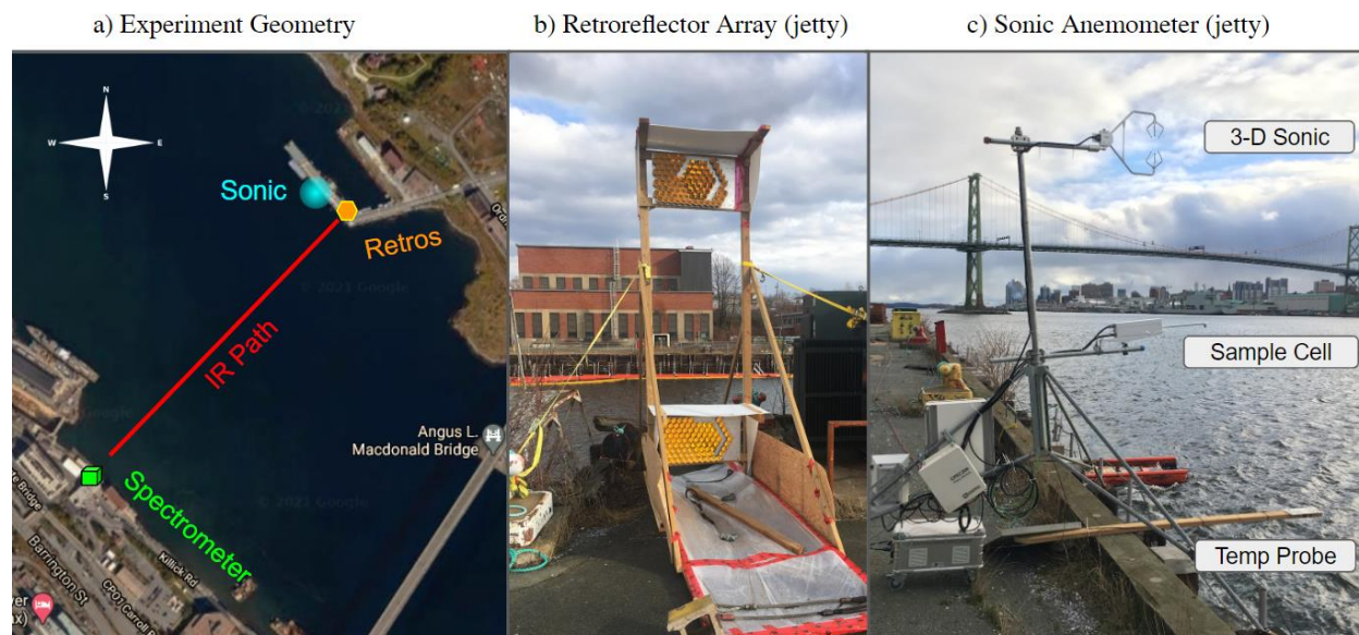
Figure 2-1: a) Layout of the experiment in Halifax Harbour. The OP-FTIR spectrometer and retroreflector arrays were connected by the 558 m IR light path. The 3-D sonic anemometer was 50 meters to the northwest of the retroreflectors on the L-shaped jetty. B) The retroreflector arrays included aluminum mounting plates for the cubes, which were fixed to a wooden structure that included plywood and plastic wind baffles, all tightly secured to anchor points that are part of the solid jetty structure c) The 3-D sonic anemometer was positioned as far over the edge of the jetty and as high as possible. The gas analyzer sample cell was used to measure barometric pressure and temperature (thermistor). A wooden beam had a temperature probe (Campbell Scientific 109; thermistor encapsulated in an epoxy-filled aluminum housing) mounted to the end out over the water.
