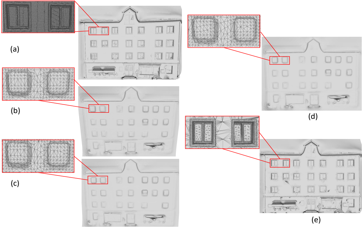
Figure 4.10: Comparison on domfountain_model (2). (a) Initial mesh model, (b) GH's method, (c) LT's method, (d) SLA's method and (e) our model.
