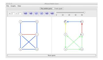
Figure 4: A snapshot of the component pebble game for 2D bar-and-joint rigidity.
