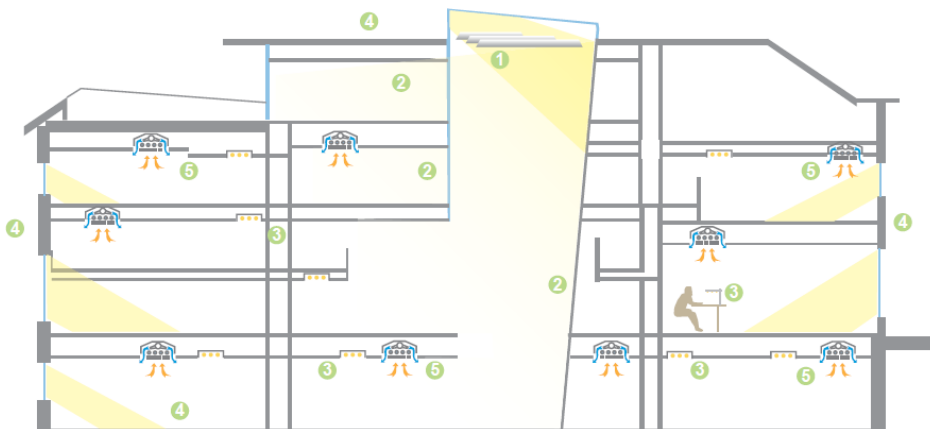
The oculus brings natural daylight into the existing building and reduces internal loads. Image Credit: Transsolar
