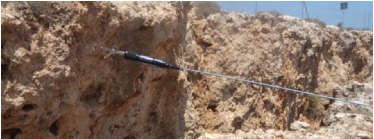
Fig. 2: The photo shows the instrument anchored at the reference pin.
