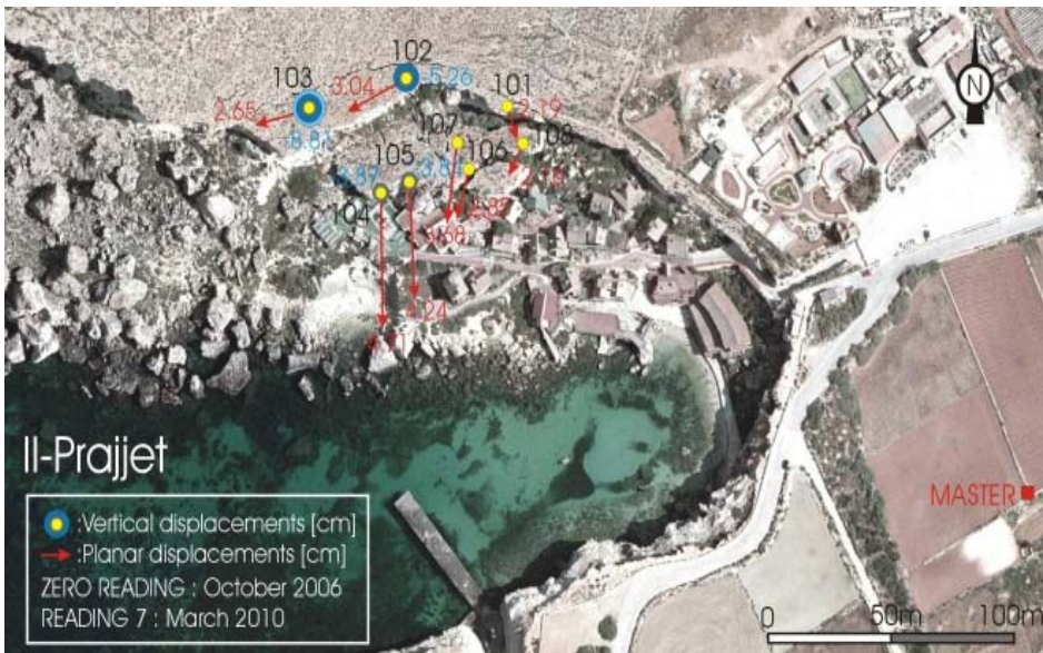
Fig. 19: Positions of the benchmarks and displacements recorded at Il-Prajjet (Anchor Bay).
