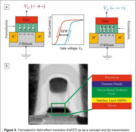
electron microscope micrograph of the FeFET cross section realized in a 28-nm complementary metal oxide semiconductor process. The different layers in the gate stack are indicated on the right.<sup>53</sup> Note: *MW*, memory window.
