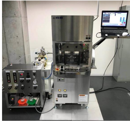
Fig. 4-13 Alpha Design TC bonder with Ar-gas atmosphere in the bonding chamber
