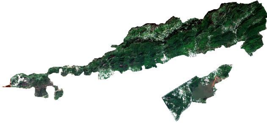
Fig. 74: Natural Colour Composite of S2 Image of the Study Area (Band combination 4,3,2)
