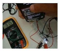
Fig. 4 - Measuring the output voltage for iPhone speaker as the source of sound energy
