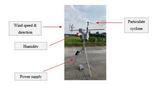
Fig. 3 - Met One E-Sampler
