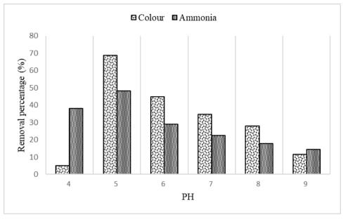
Fig. 5 - Removal percentage of colour and ammonia for AEC at different value of pH
