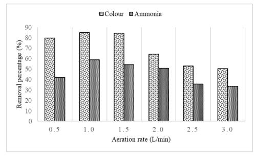
Fig. 4 - Removal percentage of colour and ammonia for AEC at different value of aeration rate
