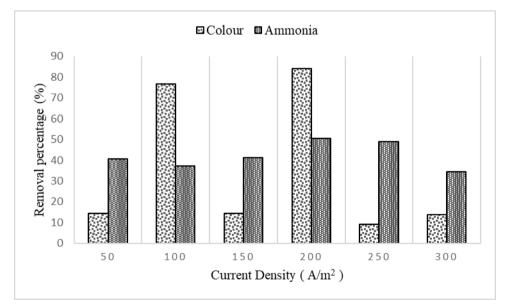
Fig. 3 - Removal percentage of colour and ammonia for AEC at different value of current density
