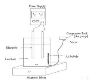
Fig. 2 - Aerated electrocoagulation process
