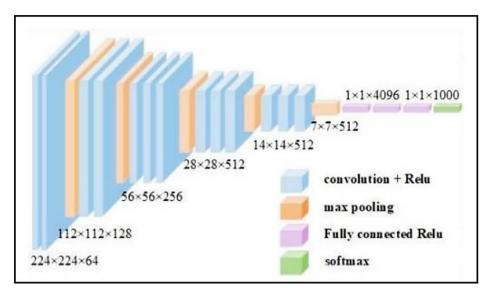
Fig. 4 - Architecture of VGG16 model [12], [13]
