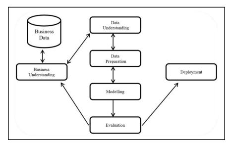
Fig. 1 - Phases of the CRISP-DM process model [10]
