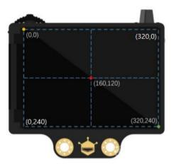
Fig. 4 - The coordinate system of HuskyLens
