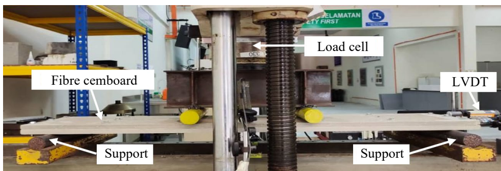
Fig. 8 - Schematic arrangement of four-point bending test
