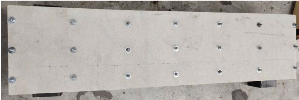
Fig. 7 - The example of bolted fibre cemboard panel
