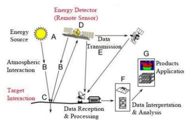
Fig. 4 - Remote sensing process [26]
