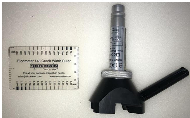
Figure 34. Crack gauge card and the handheld microscope
