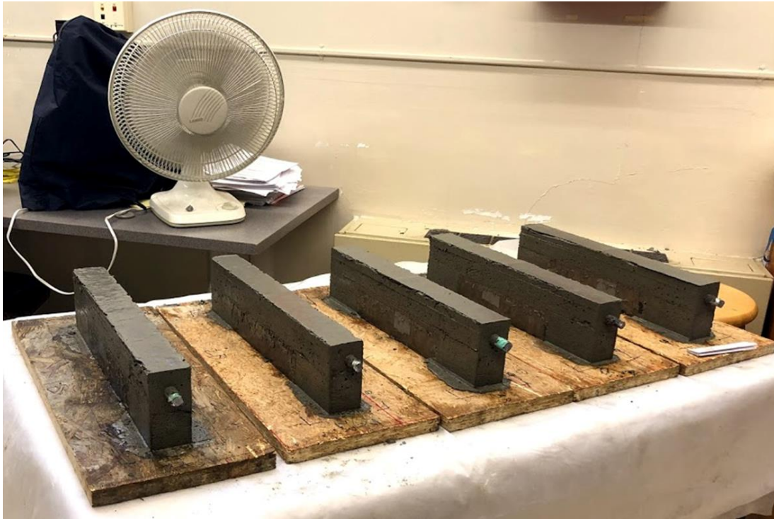
Figure 20. Shrinkage cracking test set up
