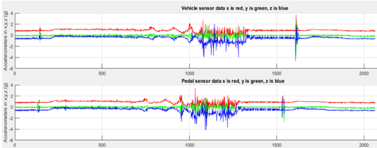
Figure 42. Accelerometer data where the x axis is red, y axis is green, and z axis is blue from the vehicle (top) and brake pedal (bottom) during a test run at 55mph in the 2012 Toyota Camry
