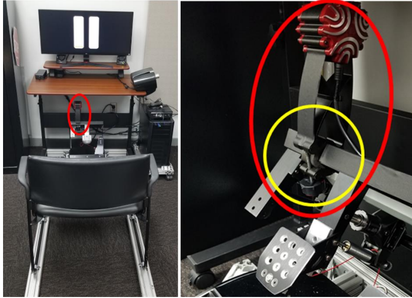
Figure 78. Simulator setup with device that delivers haptic ABS feedback circled in red (ButtKicker). The yellow circle highlights the attachment point to the pedal assembly.
