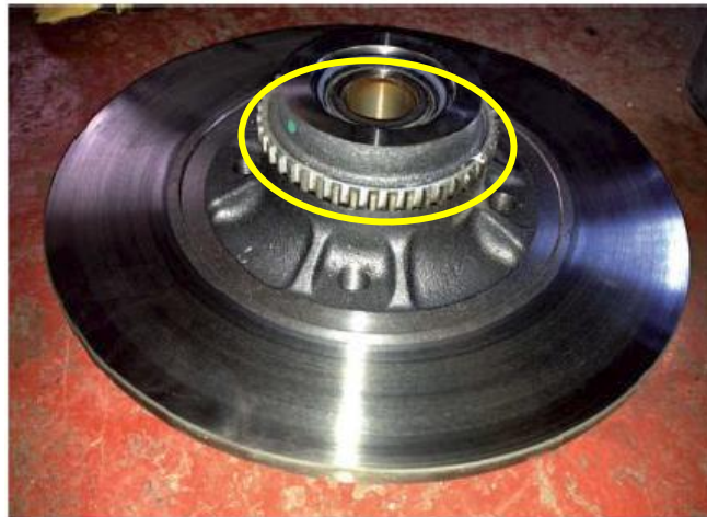
Figure 7. ABS ring (circled in yellow) on disc brake (Lawes, 2014)
