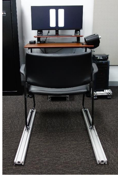
Figure 48. Chair mounted on rails to prevent tipping
