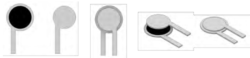
Figure 4.18: Printed sensor material layers
