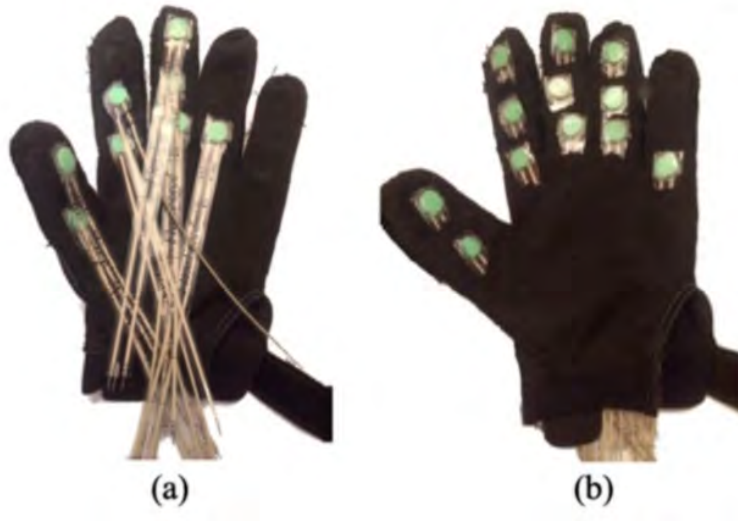
Figure 2.11: Normal force sensing glove from the research conducted by Austin et al. a) uncovered sensor lead view b) covered sensor lead view [54]
