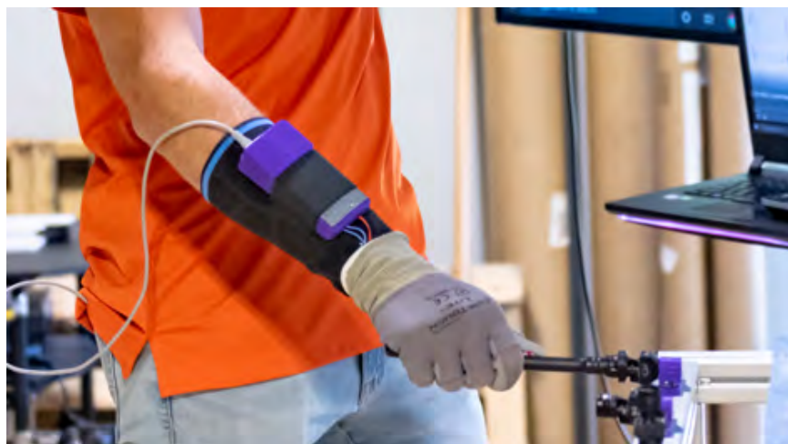
Figure 4.26: Complete sensor system used for line testing with sensor glove
