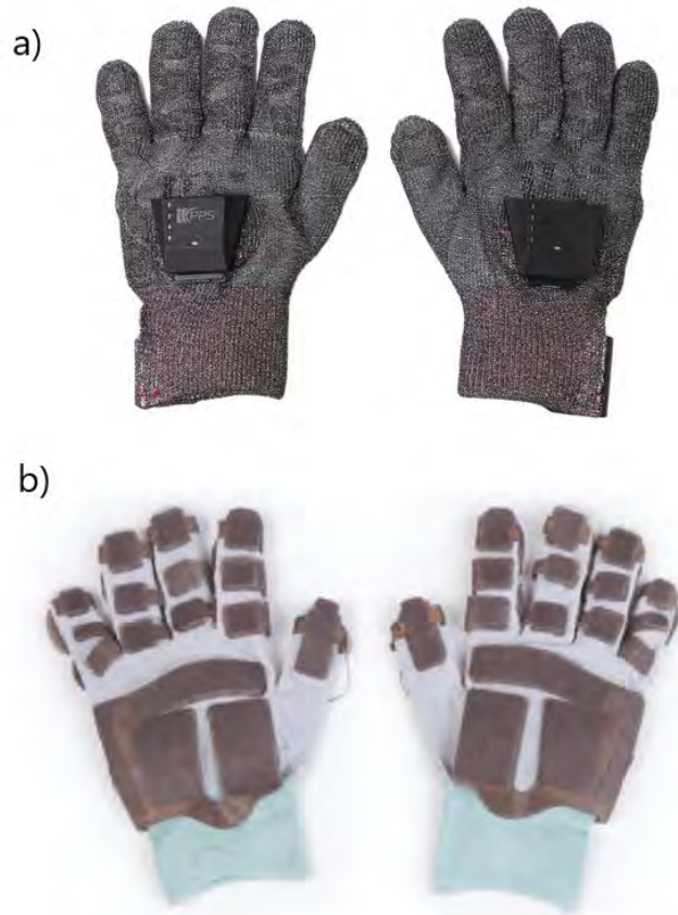
Figure 2.5: PPS TactileGlove - hand pressure and force measurement a) fully assembly glove b) inner glove lining with sensors affixed
