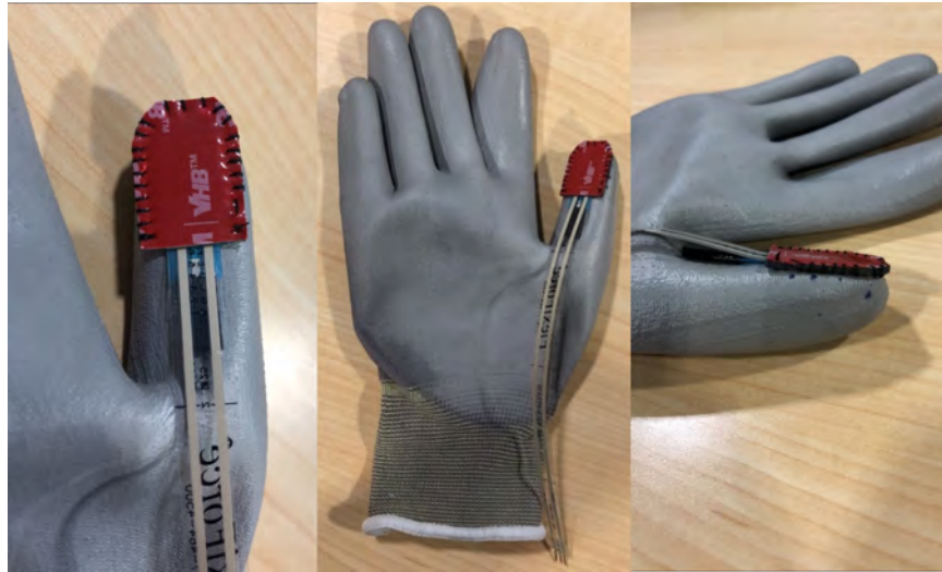
Figure 4.13: Prototype 1 of the stacked sensor affixed to the glove
