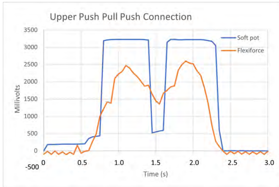
Figure 6.7: Segmented phase two - line testing completed connection example (Type 1 connector)
