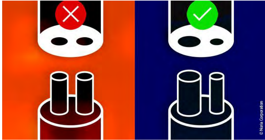
Figure 2.1: Poka-yoke principle applied to an electrical plug [21]
