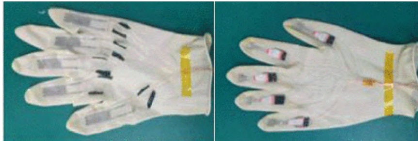
Figure 2.12: Strain sensors integrated onto the back of the finger with force sensors integrated to the finger tips from Meng et al. [55]
