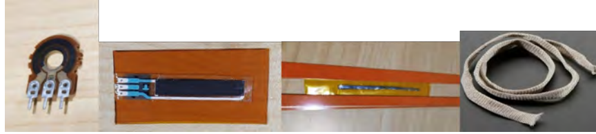
Figure 4.4: Resistive elements tested in order from left to right: rotary potentiometer, linear potentiometer, constantan foil, and conductive fabric
