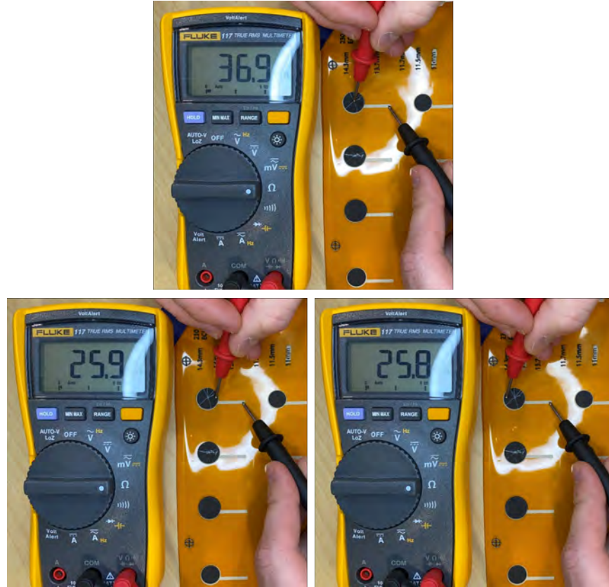
Figure 4.22: Resistive working range for printed sensor: center reading under normal force alone (top), edge reading under shear load simulating push (bottom left), and edge reading under shear load simulating pull (bottom right)
