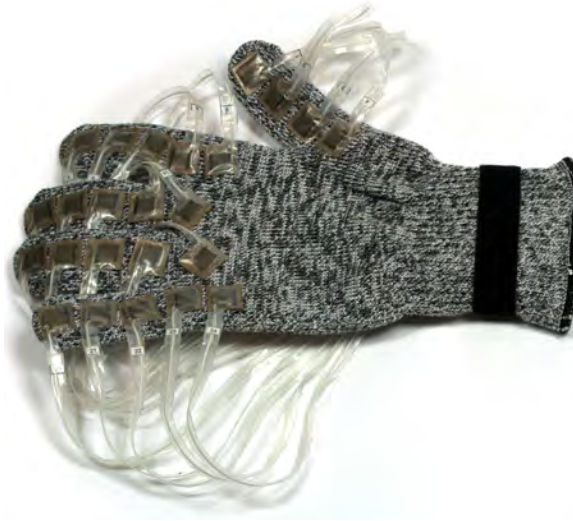
Figure 2.3: Tactilus grip pressure sensor glove with 24 sensors
