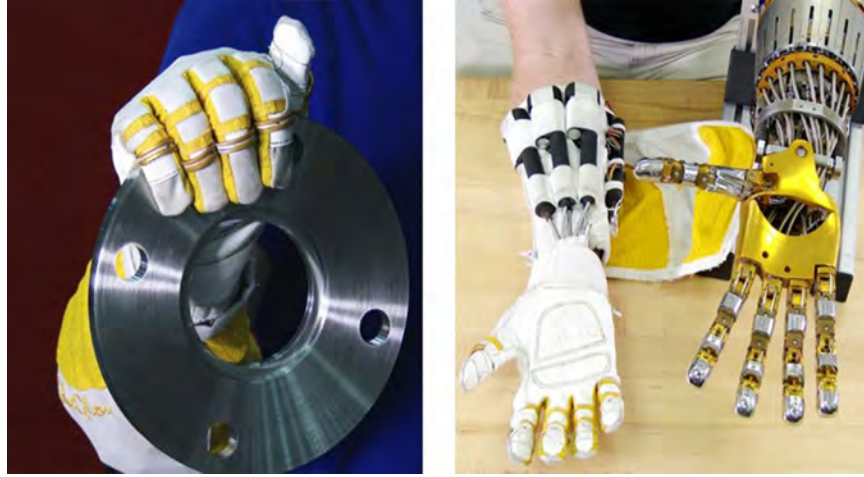
Figure 2.2: GM-Nasa Robo-Glove: Wearable technology that reduces the force needed to operate tools
