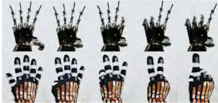
Figure 2.9: Robot hand gesturing control through sensor glove by Yin et al. [52]
