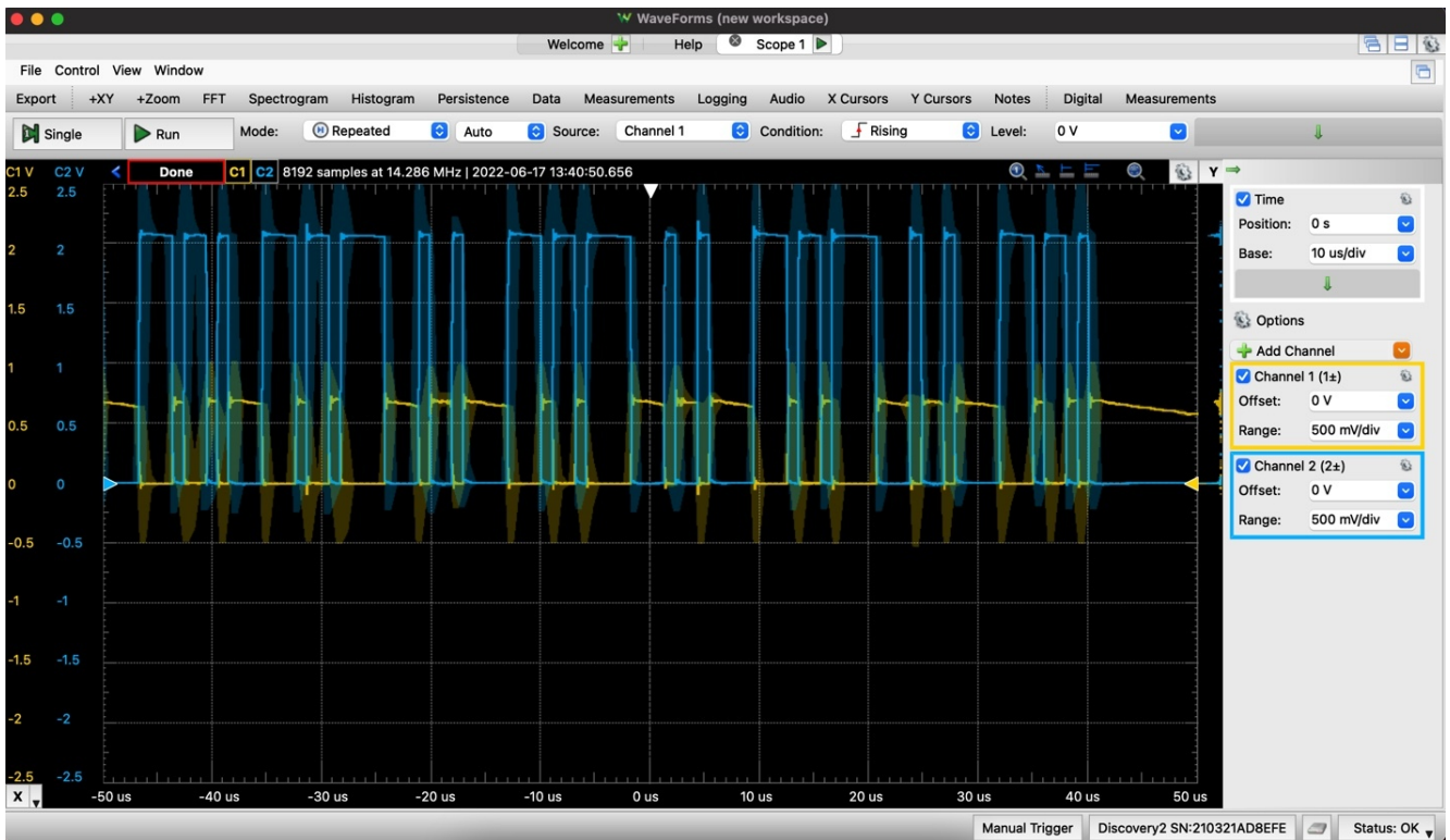
Figure 4.12: Backscattered bits from the data pin and transmitter
