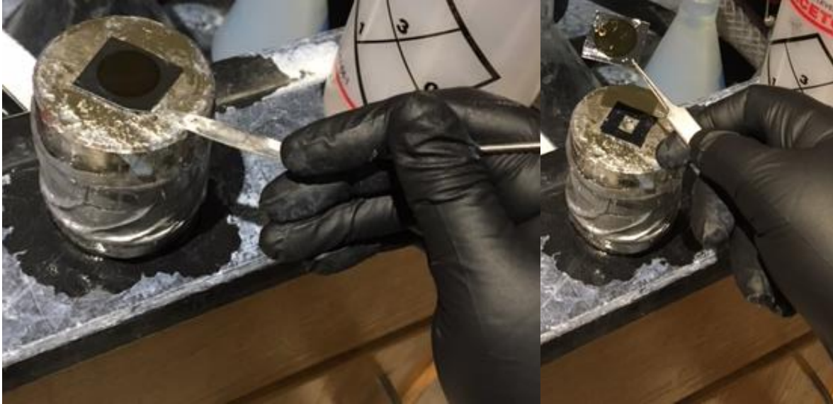
Figure S20. Removal of the sample from the chuck using the mixing spatula (left) and then forceps (right)
