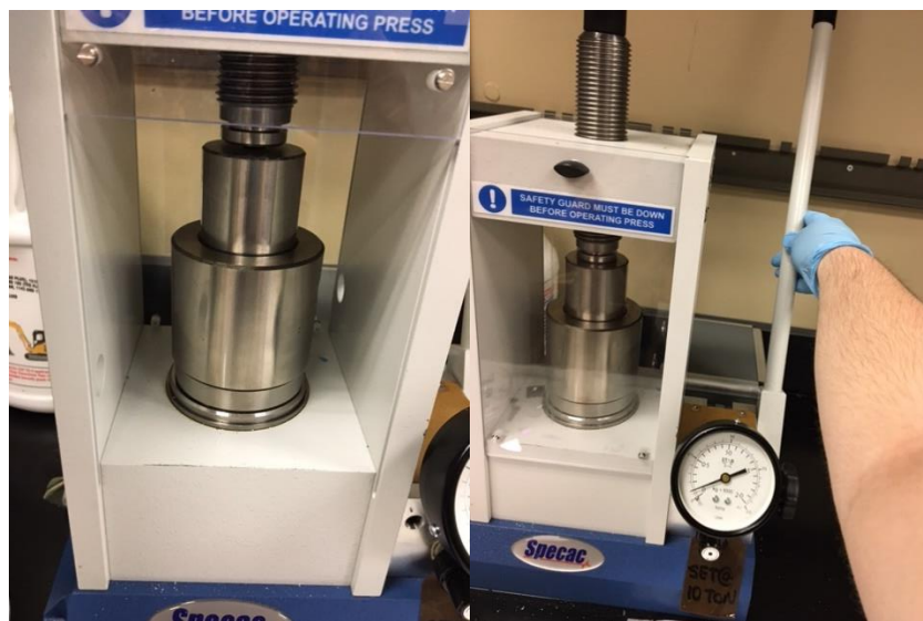
Figure S8. The jig is placed in the hydraulic press (left) and a pressure of 0.1 T is applied (right)
