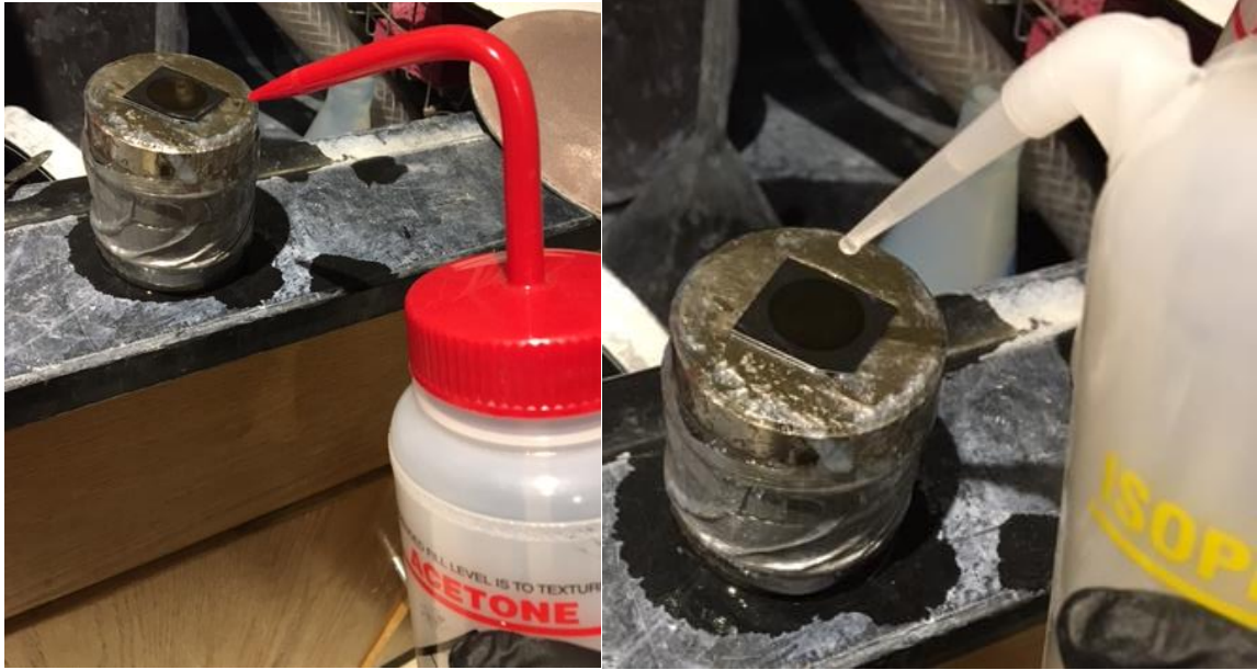
Figure S19. Acetone application (left), isopropyl alcohol re-application (right)
