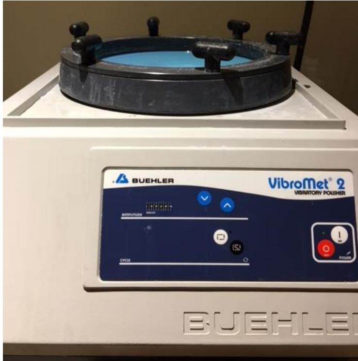
Figure S11. Buehler VibroMet 2 vibratory polisher
