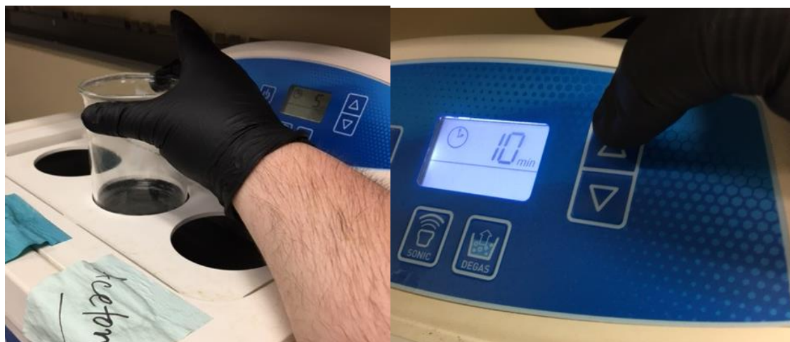
Figure S22. Isopropyl alcohol is added to a beaker (left), the polished sample is submerged in the isopropyl alcohol in preparation for sonication (right)
