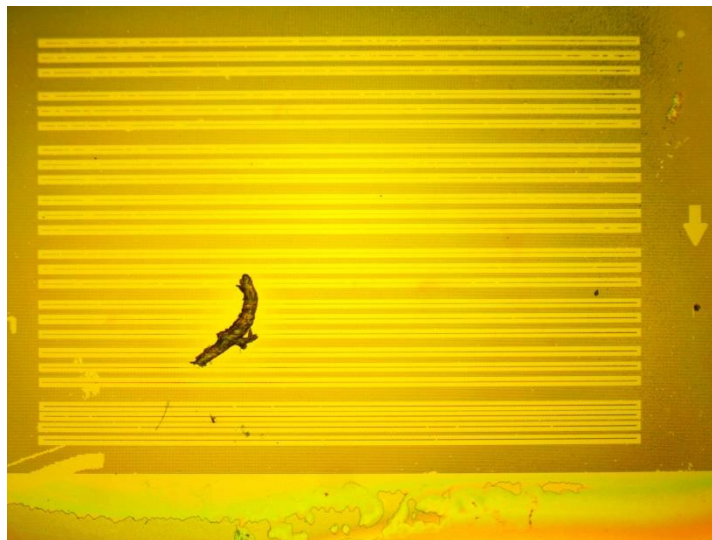
Figure S10. Microscope image showing a waveguide imprint that has been degraded by debris
