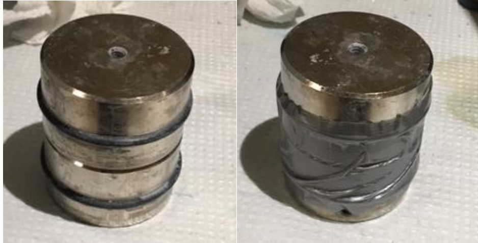
Figure S13. The chucks are stacked vertically (left) and secured with duct tape (right)
