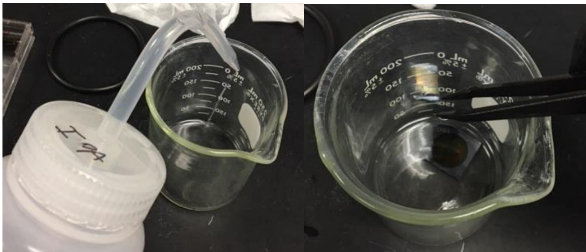
Figure S22. Isopropyl alcohol is added to a beaker (left), the polished sample is submerged in the isopropyl alcohol in preparation for sonication (right)
