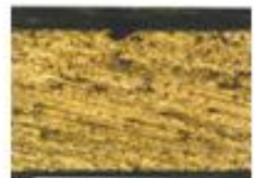
Gb 6d Penampang A-A (320x) Korosi Pitting
