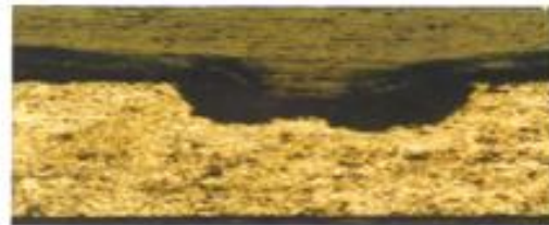
Gb.5a Penampang A-A (40x) Korosi Pitting
