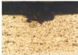
Gb 5d Penampang B-B (40x) Korosi Pitting
