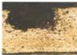
Gb 4d Penampang A-A (40x) Korosi Pitting
