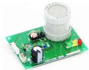
Gambar 8. Modul CDM4160 CO<sub>2</sub> (Datasheet CDM4160)
