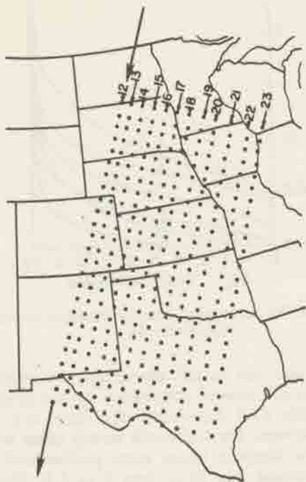
FIG. 3. VTPR scan coverage and resolution. Left half of several scan lines are shown (spots 12-23) for satellite pass over the Great Plains on 24 April 1975 at 1615 GMT.
