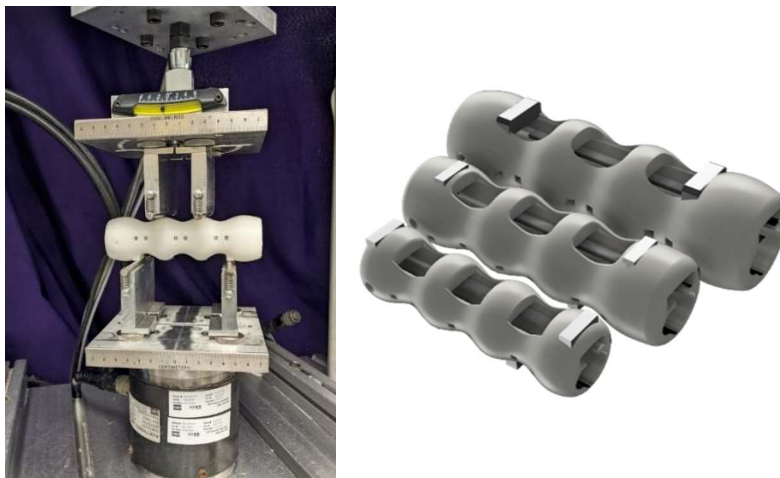
Figure 8: Design Iteration 2 loaded into the 4-point bending apparatus. 10cm, 12.5cm, and 15cm sleeves (right) were tested.
