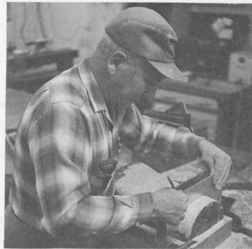
Figure 8. Modifying the wooden core for the downstream transition
