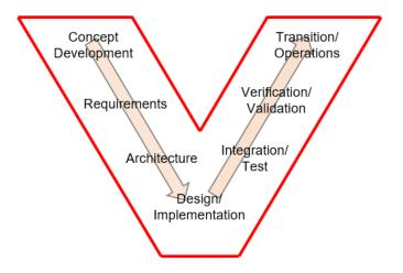
Figure 1. Systems Engineering Vee Diagram [6]
