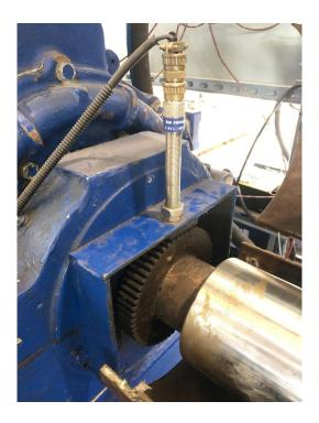
Figure 32. Dynamometer Speed Pickup
