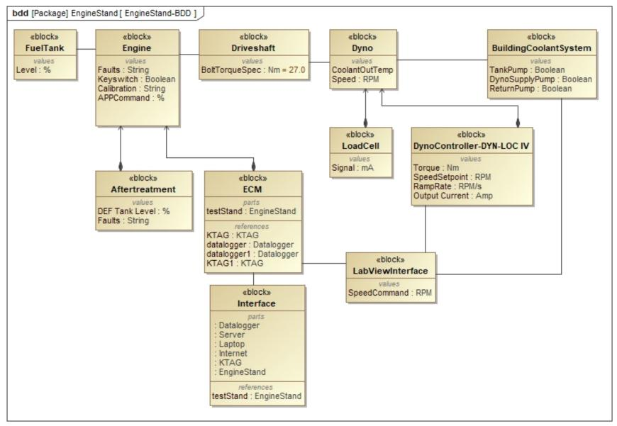
Figure 10. Engine Test Stand Block Definition Diagram
