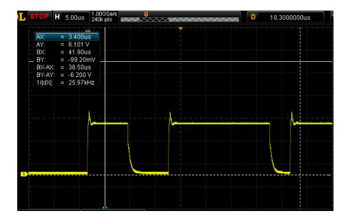
Figure 27. Oscilloscope Image of CAN high relative to CAN low: At Control Room
