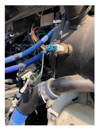
Figure 22. Kenworth Coolant Level Sensor
