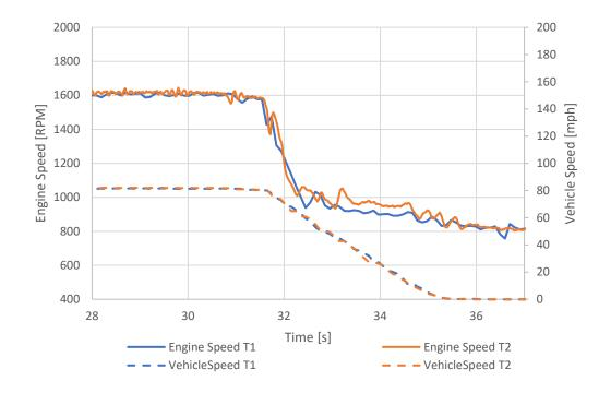
Figure 8. Engine & Vehicle Speed During Hard Brake
