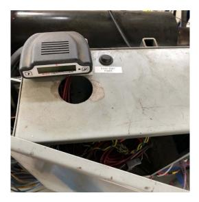
Figure 62. Diagnostic Port Power Switch
