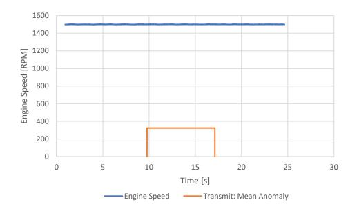
Figure 59. Engine Response to 100ms Tx: 1500 RPM with Patched Calibration
