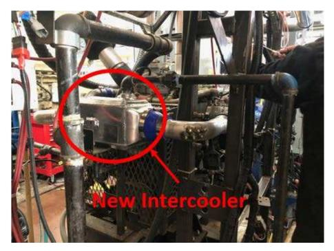
Figure 14. New Intercooler Procured and Installed
