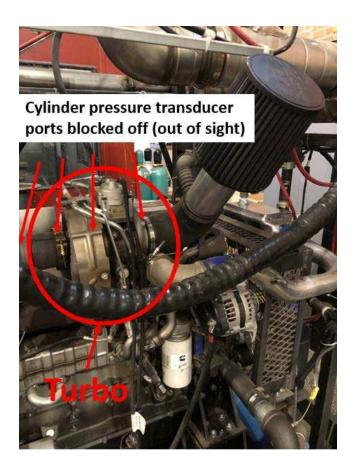
Figure 15. Cylinder Pressure Transducer Ports Blocked Off (behind turbo)
