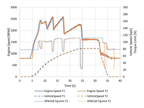
Figure 6. Kenworth T270 Hard Brake
