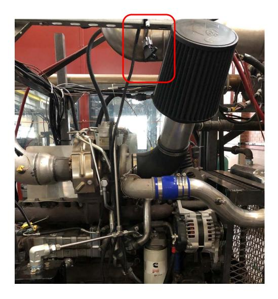
Figure 19. Ambient Air Sensor
