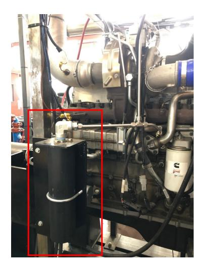
Figure 46. Turbocharger Oil Accumulator
