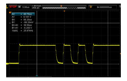
Figure 26. Oscilloscope Image of CAN high relative to CAN low: At Engine
