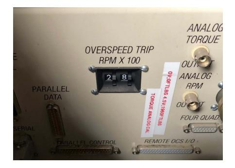
**Figure 45. Dynamometer Overspeed Protection**
