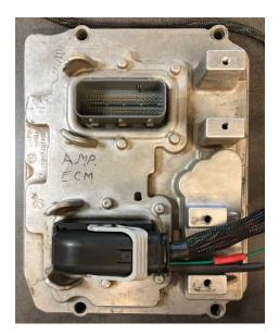
Figure 40. CM2350 with Wiring Harness
