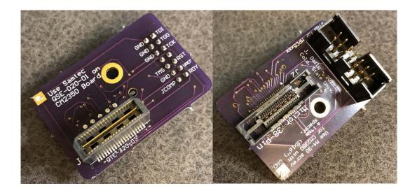
Figure 36. Custom JTAG Connector Board
