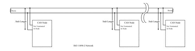
Figure 24. CAN Bus Physical Architecture [17]
