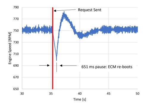
Figure 57. Engine Response to Single Tx: Idle
