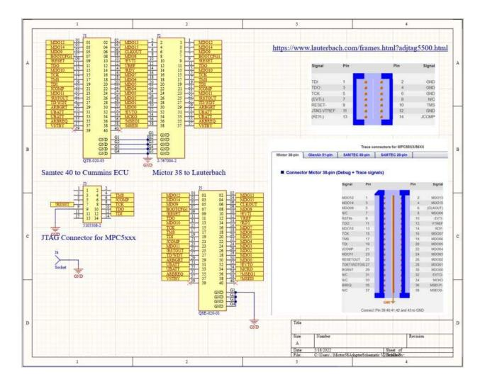
Figure 37. Custom JTAG Connector Board Schematic
