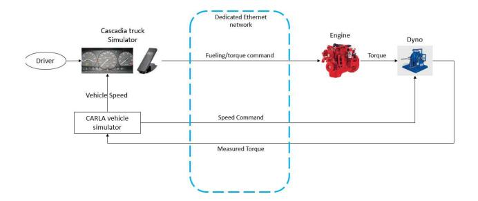
Figure 65. Potential Hardware-In-The-Loop Architecture
