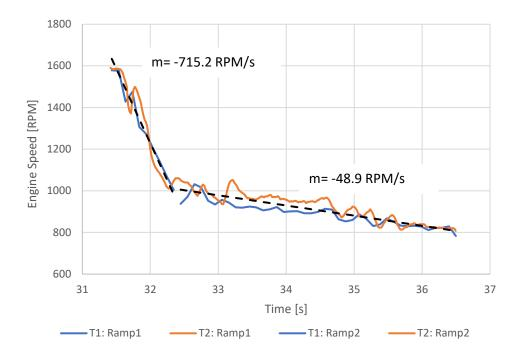
Figure 9. Piecewise Engine Ramp Rate
