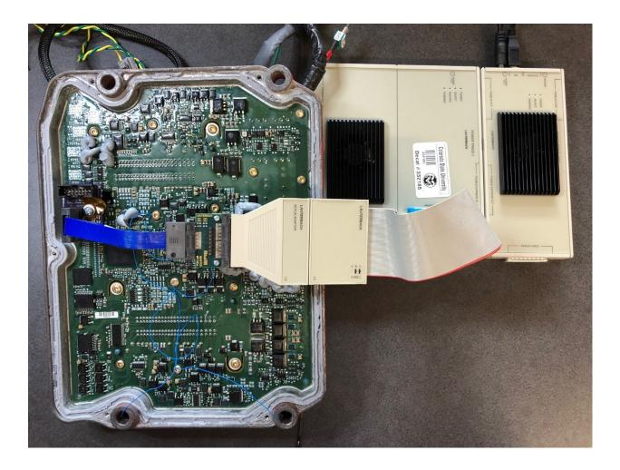
Figure 63. Lauterbach PowerTrace II Connection to CM2350
