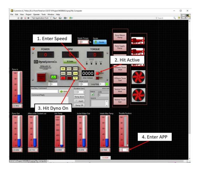
Figure 61. LabVIEW Screen: Operating Engine
