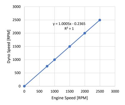
Figure 33. Dynamometer Speed Calibration
