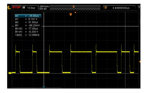
Figure 25. Oscilloscope Image of CAN high relative to CAN low: At Engine with Tether Disconnected
