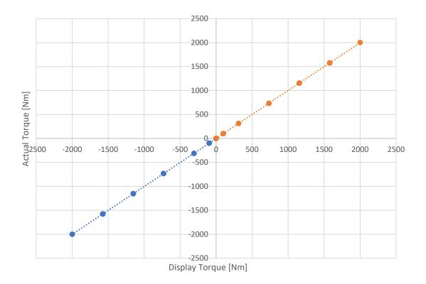
Figure 31. Load Cell Calibration Curve
