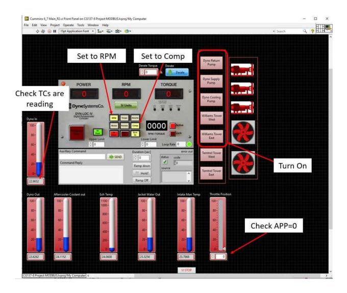
Figure 60. LabVIEW Screen: Pre-Test Checks
