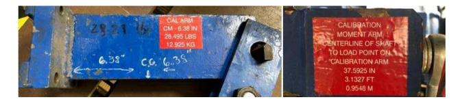
Figure 30. Calibration Arm & Load Cell Moment Arm Dimensions
