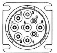
Power to pin B in on the round diagnostic connector was run through a small rocker switch mounted on top of the test stand's electrical box shown in Figure 62. This is useful for leaving data loggers on for an extended period of time provided external power is supplied to the test stand's batteries.
