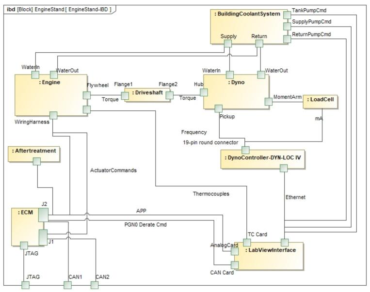
Figure 11. Engine Test Stand Internal Block Diagram
