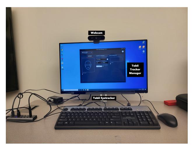
**Figure 3.1:** Computer monitor set up. The eyetracker is mounted to the bottom of the monitor using a magnetic support strip. The Camera is mounted to the top only using the camera's built in clamp. The Tobii Eyetracker manager program handles the calibration and monitor set up
