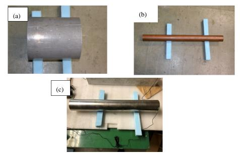
Figure 5. Setting of standard materials for EWV measurement, (a) Al, (b) Cu and (c) austenitic stainless steel (SUS304).
