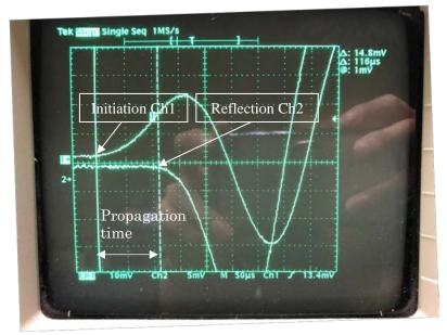
Figure 4. Example of elastic wave measurement in concrete pile Time 50µs/div. Ch1 10mV/div. Ch2 5mV/div.
