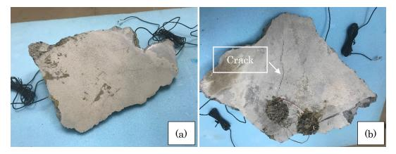
Figure 7. Concrete test pieces crashed by the steam pressure cracking agent, (a) piece having approximately 300 mm length without cracks, (b) piece having approximately 400 mm length with cracks.
