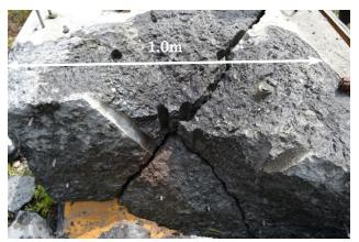
Figure 1. Reinforced concrete cut with SPC
