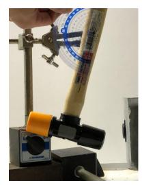
Figure 3. Alignment of the hammer impact method
