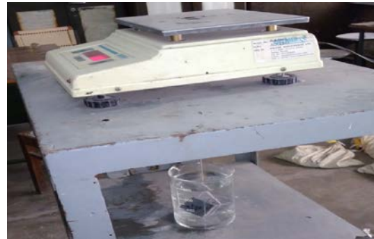
Fig. 5. Determining submerged weight
