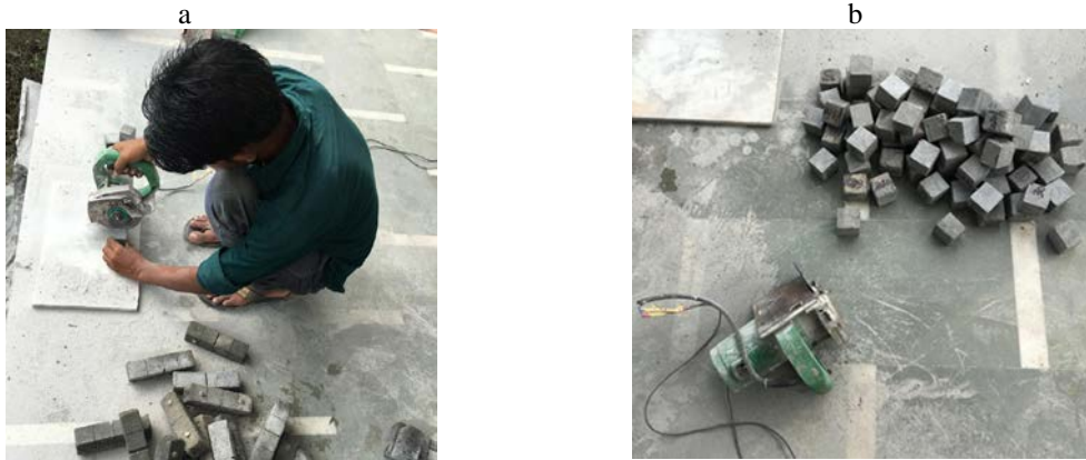
Fig. 3. (a) Cutting of flexure specimens; (b) Cubical specimens (40 mm 3 ) for compression testing.
