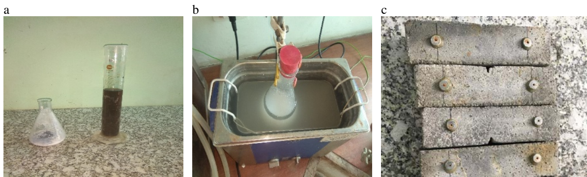
Fig. 1. (a) NS and CNTs mixed with water and superplasticizer; (b) Sonication for proper mixing of NS and MWCNTs; (c) Casted flexural specimens before testing.
