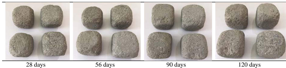
Fig. 13. Cubical specimens (T2) after Los Angeles abrasion testing
