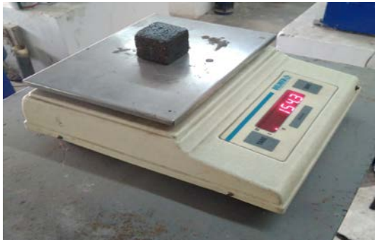
Fig. 4. Determining dry and saturated weight
