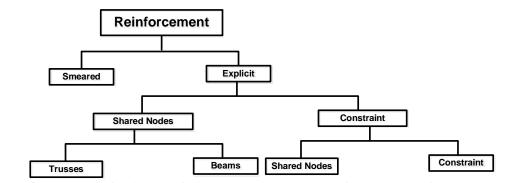
Figure 3. Schematic of various reinforcement modelling methods for rebar in reinforced concrete [26]
