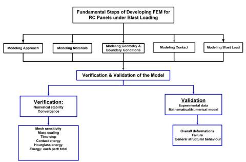
Figure 1. Effective FEM procedure for RC Panels Subjected to Blast Load
