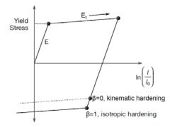
Figure 2. Elastic-plastic behaviour with kinematic and isotropic hardening (LSTC 2017b[24])
