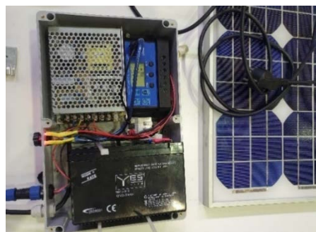
Figure. 2. Power supply system feeding the proposed DAQ
