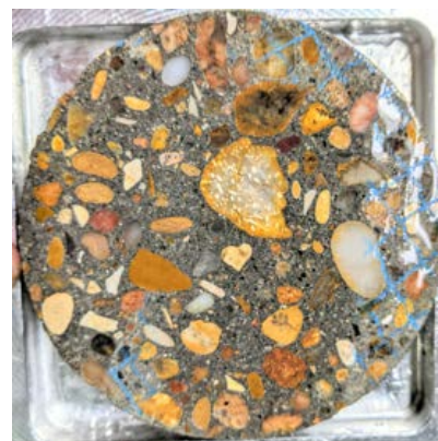
Figure 4. Example of the drawn grid with crayon. Figure 5. Example of an incomplete polish.
