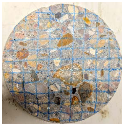
Figure 4. Example of the drawn grid with crayon. Figure 5. Example of an incomplete polish.
