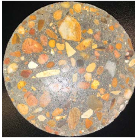
Figure 3. Diamond blade cut quality.
