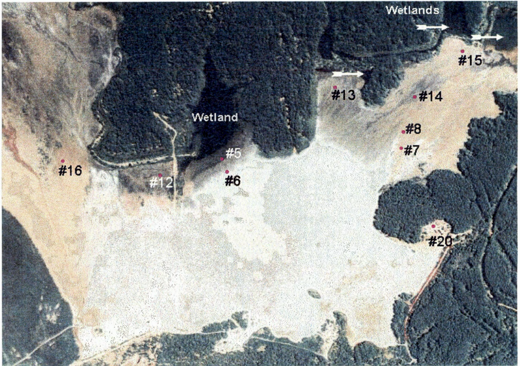
Figure 6. Aerial map of mine tailings pond showing location of cores in relation to wetlands.
