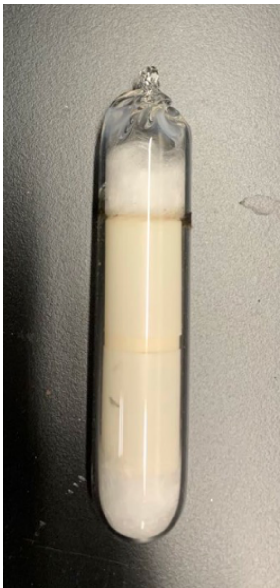
Figure 2.1: A sealed quartz tube use for flux growth. A set of crucible is put inside. Chemicals were placed inside the crucible set. Quartz wool was placed on both end inside the tube to prevent form breaking.
