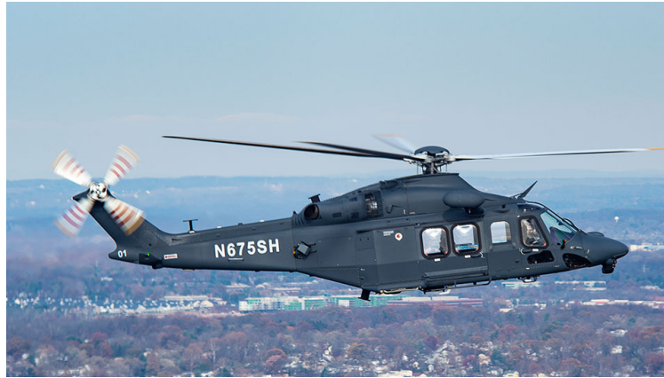
Figure 13: Boeing MH-139A with “beanie” hub fairing [106]
