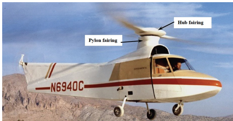
Figure 12: Lockheed CL-475 with pylon and hub fairing [4]
