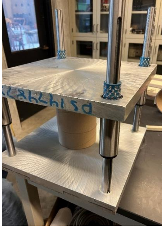
Figure 32 Die set that the test apparatus is built up around
