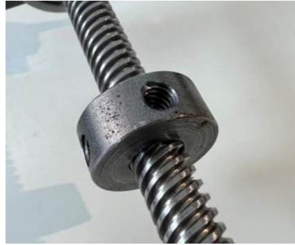
Figure 42 Fabricated flywheel hub
