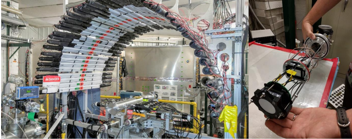
Figure 9: Experimental setup at the NSCL. (Left) Above the beamline, 42 VANDLE modules are arranged in a cylindrical arc. An array of close-packed gamma ray detectors are placed below the beamline. (Right) Within the beamline is the position-sensitive implant detector and scintillator that serves as a light ion veto.
