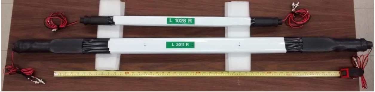
Figure 11: Assembled small and medium VANDLE modules.
