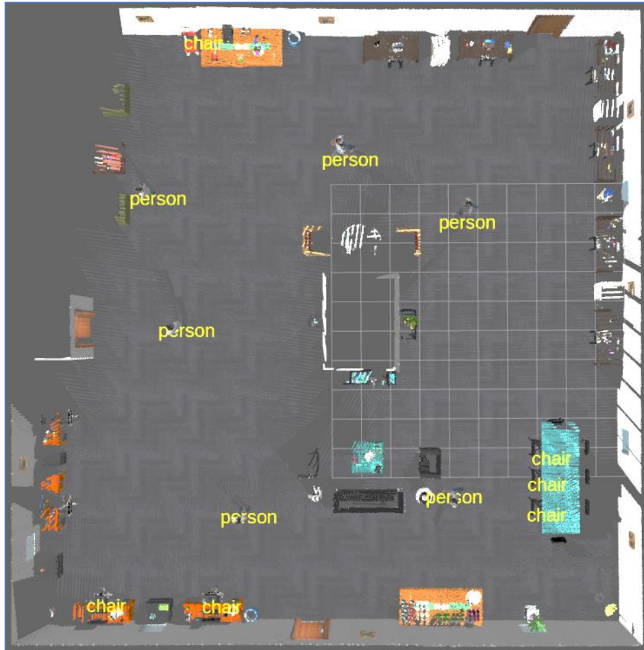
Figure 3.15. Reconstructed 3D map with object information in the simulation platform
