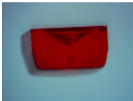
Figure 2.1.1. A) Side profile of FAPbBr 3 grown in a vial with a curved bottom showing significant concavity, B) Smooth crystal surfaces after growth
