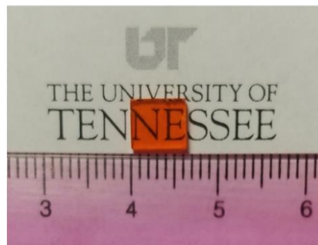
Figure 2.1.1. A) Side profile of FAPbBr 3 grown in a vial with a curved bottom showing significant concavity, B) Smooth crystal surfaces after growth
